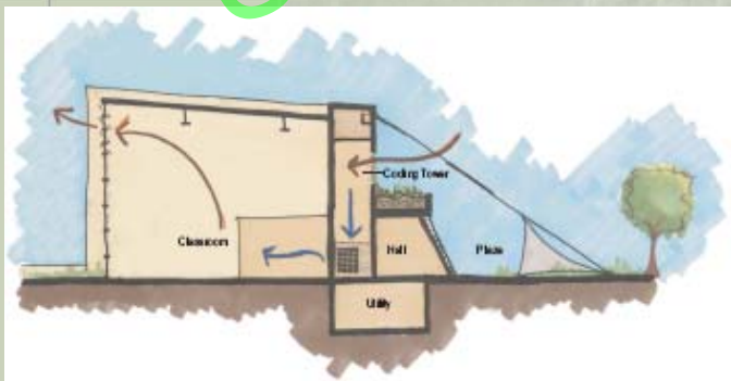
(A) Section at Cooling Tower 1/8" = 1/4"
